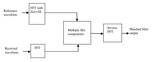
Figure 1.7: Digital matched filter correction processor
