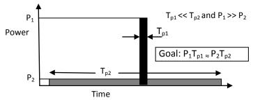
Figure 1.4 illustrates two pulses having same energy with different pulse width and peak power
